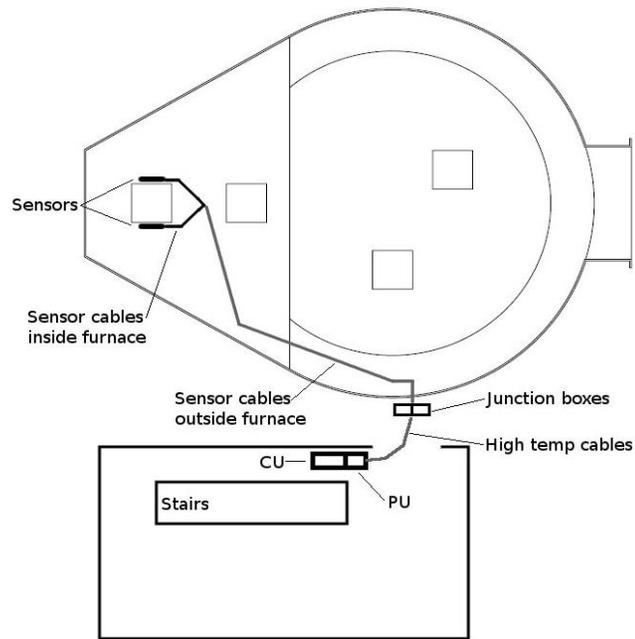
**Figure 4 Installation layout**
