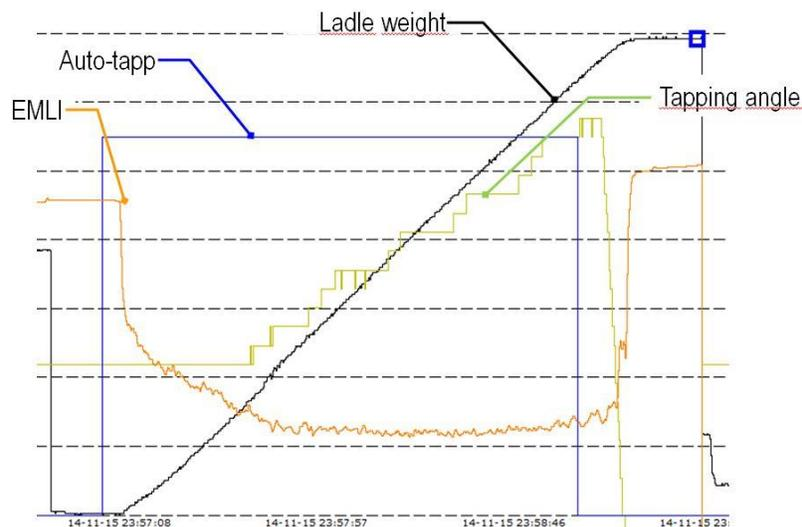
**Figure 5** Signals recorded during tapping: (Heat No. 143900)
