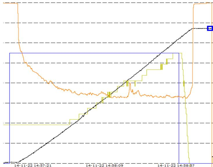
**Figure 6 Tapping with slag entrainment midway**
