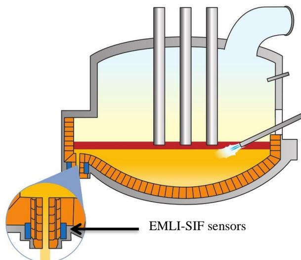
**Figure 1 EMLI-SIF Sensor position on two sides of the tap hole**
