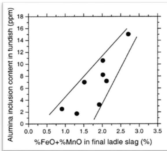
Figure 4: The effect of %FeO+%MnO content on the amount of alumina inclusions<sup>[3]</sup>.
