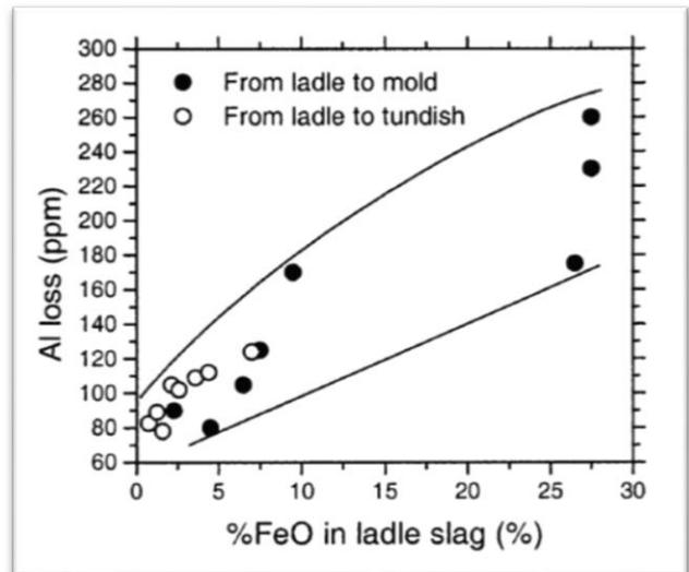
Figure 3: The loss of aluminum as a function of FeO-content in ladle slag<sup>[3]</sup>.
