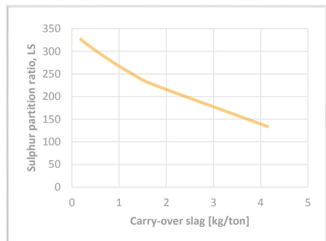
Figure 5: The effect of slag carry-over from electric arc furnace on the sulphur partition ratio.
