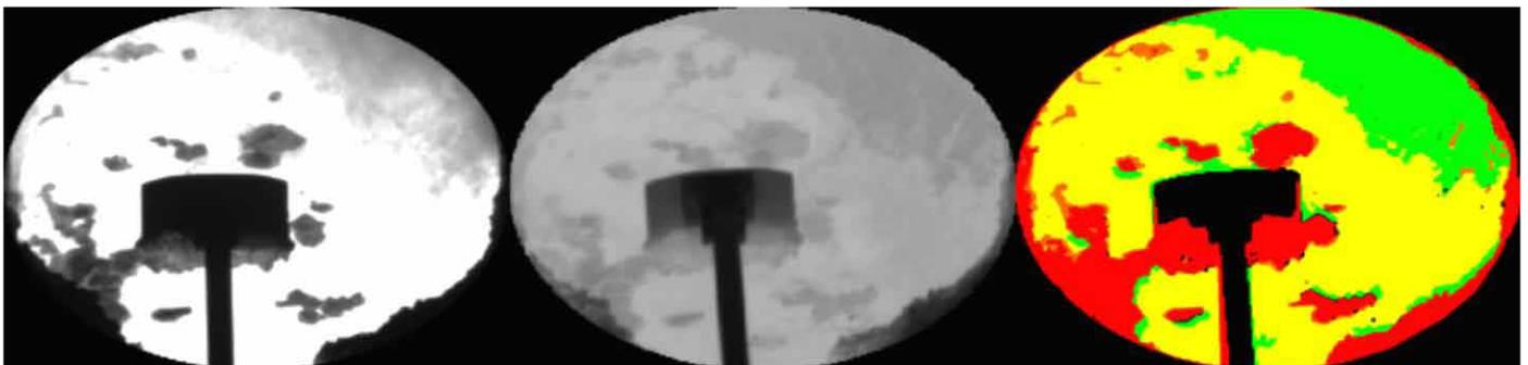
Figure 7: Example of video frames showing the near infrared image (left), infrared image (center) and analyzed output (right). The analysis output codes thick slag as red, thick liquid slag as orange, thin slag as yellow and free metal surface as green.
