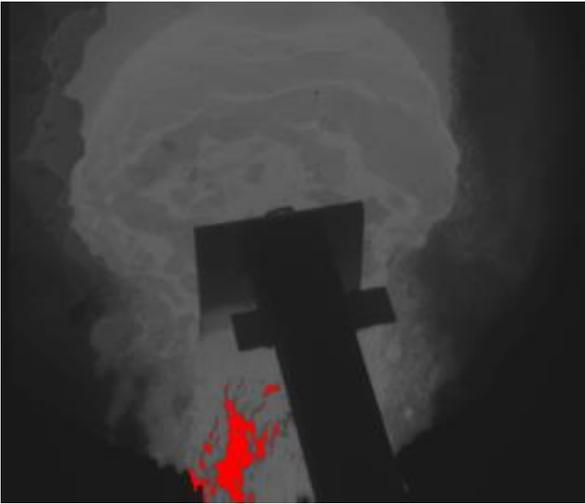
Figure 1: Metal losses (marked by red) during ladle deslagging as interpreted by vision analysis.
