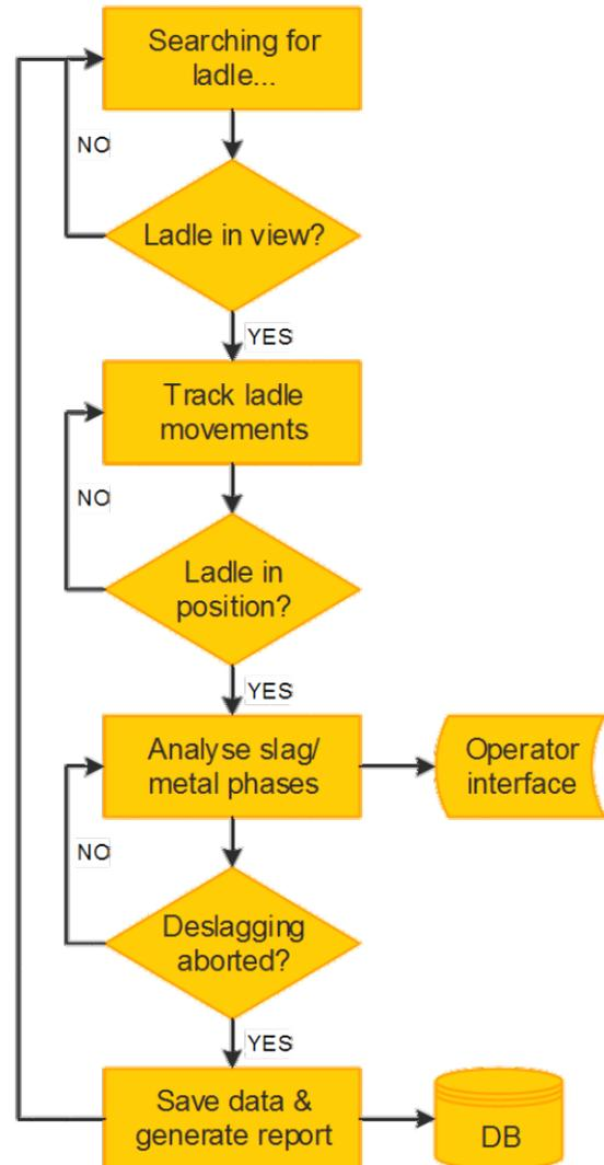
Figure 6: Basic principle of LadleSlag analysis.
