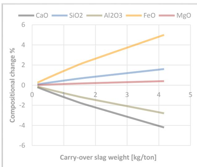
Figure 2: Relative compositional change of synthetic slag due to slag carry-over from electric arc furnace.
